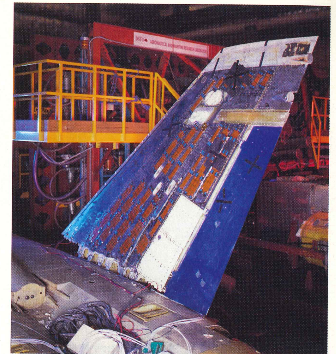
Figure 12. ACX custom-designed QuickPack actuators installed on one vertical tail surface of an F/A-18 airframe. The IFOSTP ground vibration test rig is seen in the background. (Photo courtesy of AMRL.)
