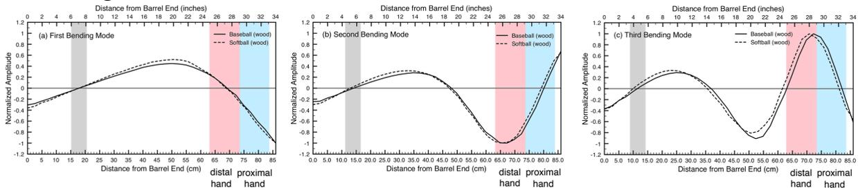
Fig. 3 – Mode shapes and frequencies for the first three bending modes of a typical composite field hockey stick, showing hand locations.
