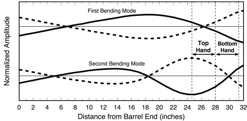
**Fig. 1.** Mode shapes for the first two bending vibrational modes in a 32-inch youth baseball bat. Barrel end is at the left and handle is at the right.
