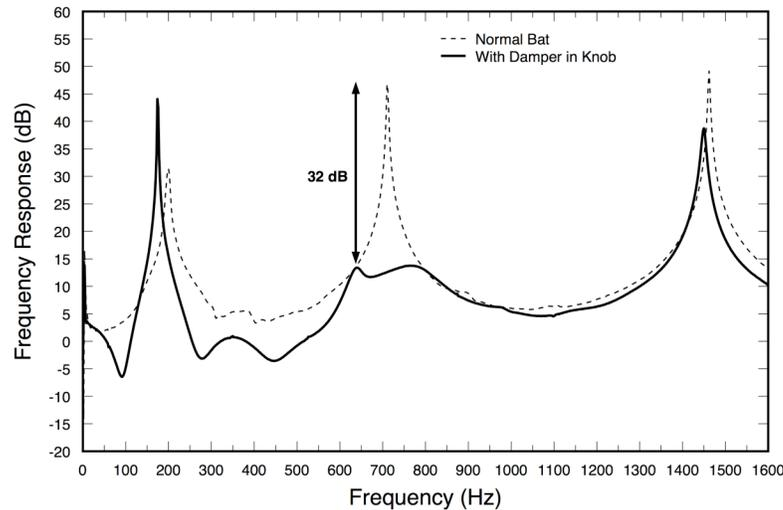
**Fig. 2.** Frequency response function for a baseball bat with a tuned-mass damper in the knob. Tuning the damper to the frequency of the second bending mode effectively removes that mode from the resulting vibration of the bat.
