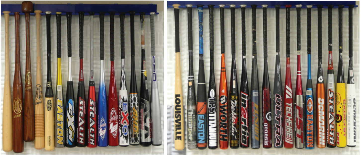
Figure 1. Examples of the variety in baseball and softball bat construction. Left: Baseball bats. Left to right: pro-stock wood, replica of Heinie Groh's wood bottle bat, large knob wood bat for swing training, wood with composite coating, two piece with aluminum handle and laminated bamboo barrel, single-piece aluminum, two-piece aluminum, two-piece stiff composite handle with aluminum barrel, two-piece flexible composite handle with aluminum barrel, single-piece composite, composite with double-walled barrel, composite with very stiff handle, aluminum with vibration absorber in knob, aluminum with electronic vibration dissipation circuit on handle, and aluminum with aerodynamic holes in taper. Right: Softball bats. Left to right: wood, 1972 single-walled aluminum, 1993 graphite, 1993 titanium, single-walled aluminum, double-walled aluminum, triple-walled aluminum, two-piece composite handle with aluminum barrel, composite, composite high performance, multiwall (aluminum exterior with composite inner shell), high-performance aluminum double-walled barrel, two-piece antivibration joint with aluminum handle and triple-walled aluminum barrel, two-piece composite handle with aluminum double-walled barrel, two-piece composite handle joined to composite barrel, two-piece stiff handle with composite barrel, and two-piece composite handle with steel single-walled barrel.
