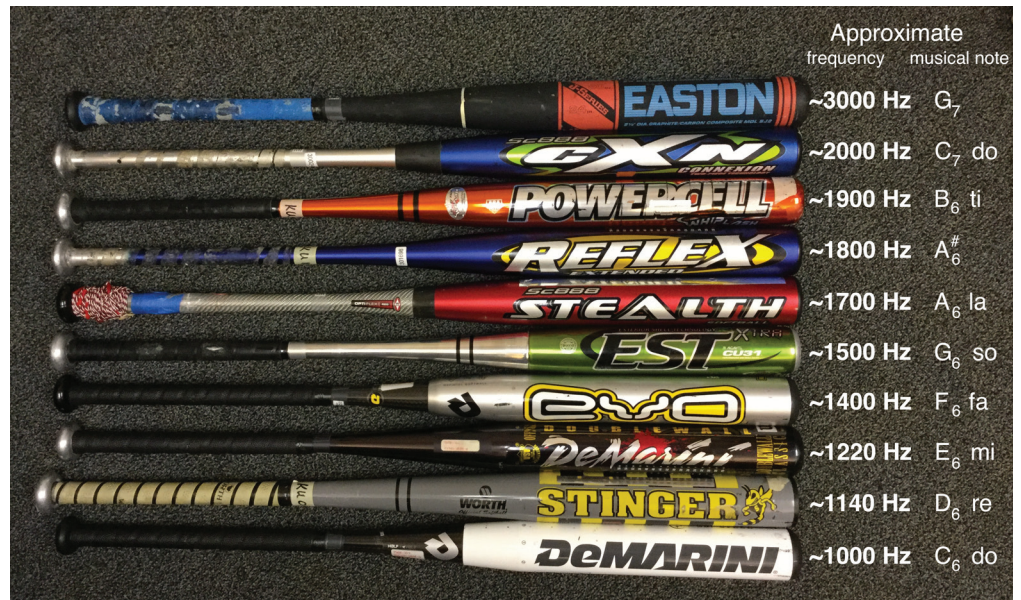
Figure 7. A selection of softball bats with hollow metal or composite cylindrical barrels having hoop frequencies that form a good approximation of a musical scale. This “bat piano” can be used to play tunes (Video 4 at http://acousticstoday.org/russell-media ).
