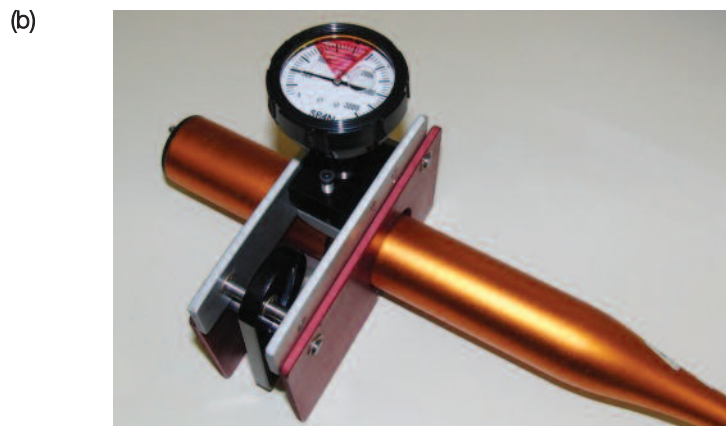
Figure 3. Barrel compression testers measure barrel stiffness of hollow composite or aluminum softball bats: (a) setup for laboratory testing and (b) portable device.
