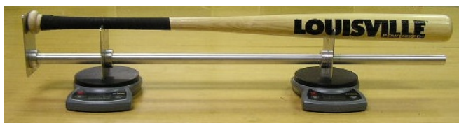
Fig. 3. Apparatus for measuring the weight and balance point of a softball or baseball bat.
