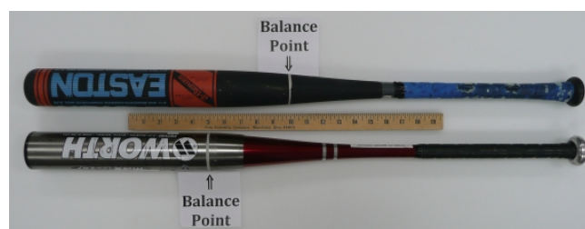
Fig. 1. Two slow-pitch softball bats of the same length and weight, but very different balance points (centers-of-mass).
