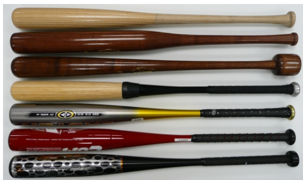
Fig. 5. Wood, aluminum, and composite adult baseball bats with different profiles, corresponding to data in Table II.
