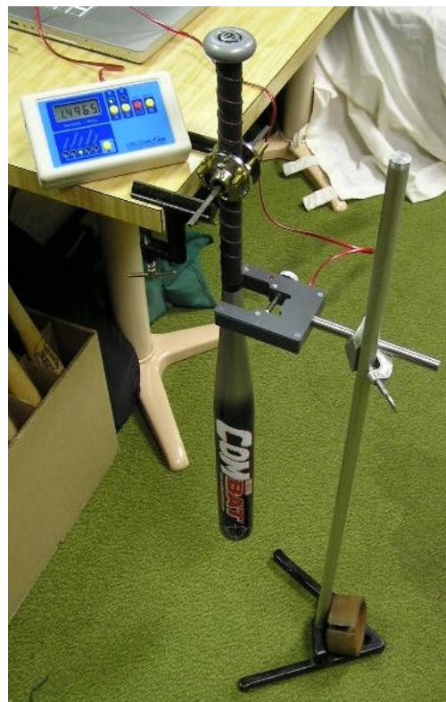
Fig. 4. Apparatus for measuring the period of oscillation for a softball bat pivoted about a point 6-inches from the end of the handle.
