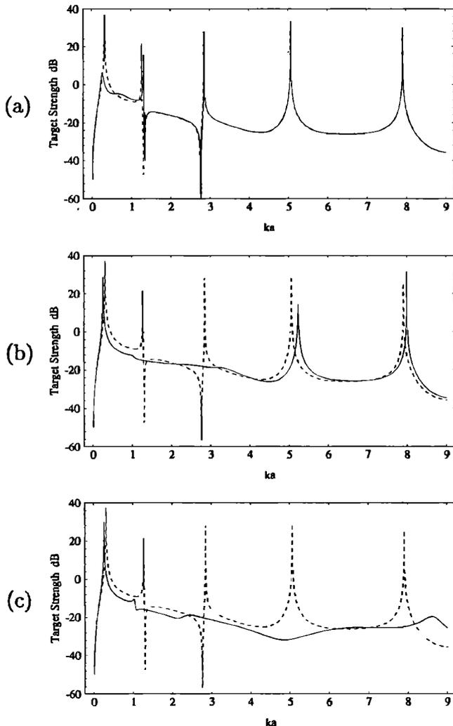
FIG. 5. The dashed curves represent the target strength at  $45^\circ$  for the plate without any attachments. The solid curves represent the target strength at  $45^\circ$  for the plate with fuzzy attachments. The total mass of the fuzzy attachments is 40% of the plate mass. (a)  $K_F a = 0.316$ , (b)  $K_F a = 1.265$ , (c)  $K_F a = 2.846$ .
