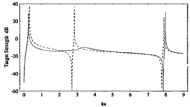
FIG. 6. A comparison between the backscatter from the plate with (solid curve) and without (dashed curve) attachments for normal incidence. The total mass of the attachments is 40% of the plate mass, and  $K_F a = 1.265$ .
