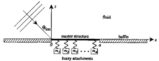
FIG. 1. Plate strip with internal fuzzy attachments, simply supported in an infinite baffle.
