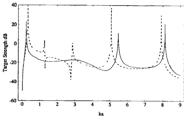
FIG. 7. Dependence of target strength on total mass of attachments: (dashed) total mass of attachments is 1% of plate mass; (solid) total attached mass equals plate mass.  $K_F a = 1.265$ .
