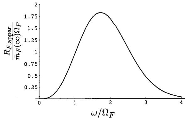
FIG. 4. Normalized apparent damping constant added to the plate strip by the fuzzy attachments, in the limit  $\zeta \rightarrow 0$ , when the plate is vibrating with frequency  $\omega$ .
