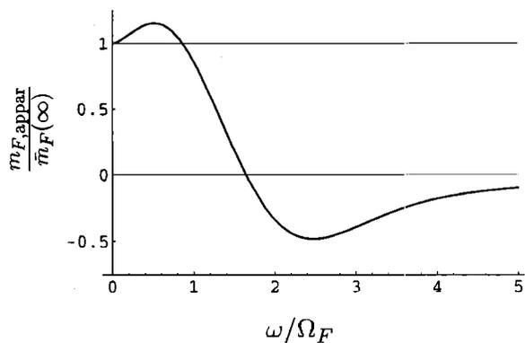
FIG. 3. Normalized apparent mass per unit area added to the plate strip by the fuzzy attachments, in the limit  $\zeta \rightarrow 0$ , when the plate is vibrating with frequency  $\omega$ .
